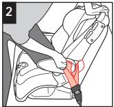
Place one knee in the child restraint and push down firmly while pulling up on belt to tighten. For a manual belt, refer to "Knowing your Vehicle Belt" section.
